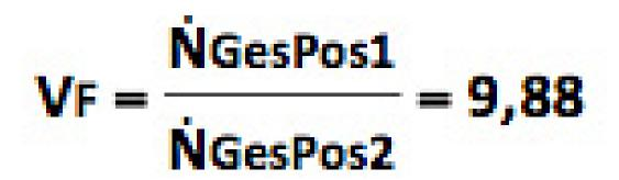
Provided the first measurement is not affected by a coincidence error and the dilution system under test is working (not soiled), a dilution factor of almost 10 is determined. If this should not be the case, there was possibly a coincidence in measurement 1. In this case, the aerosol concentration has to be decreased or a further dilution step used. Another possibility would be that the dilution step to be tested is soiled. In this case, the device has to be cleaned and the test repeated.
