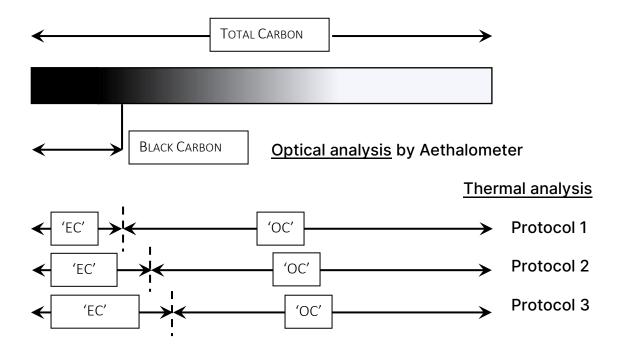
Thermal analysis methods usually agree quite well with each other for the determination of the Total Carbon content of the sample: but there may be substantial differences in the "EC/OC" partitioning, depending on the nature of the sample and the thermal protocol which is used for analysis.
