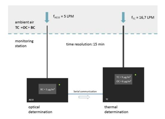
The TC and BC data are combined to yield the OC result by simple subtraction.
