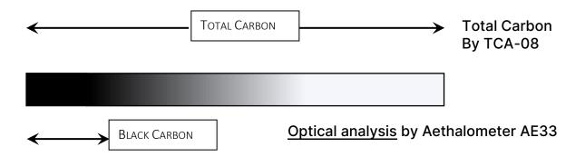
Multiply BC by 1.3 to estimate "IMPROVE EC": subtract from TC to derive 'OC'.
